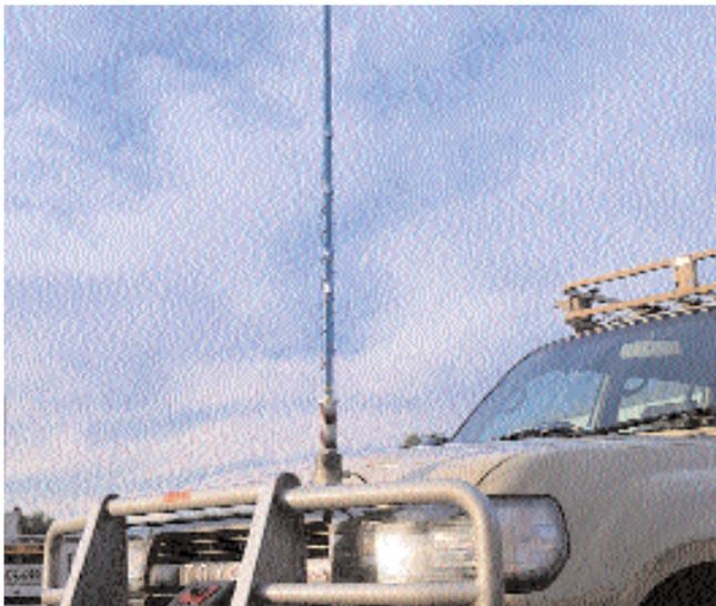
Only one long range antenna (large diameter base) may be fitted to the front of a vehicle and must be fitted to the left side. The maximum diameter permitted is 75mm.
